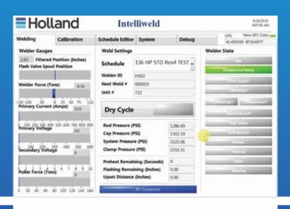
The Intelliweld® Control system is Holland's proprietary welding system and the next generation in our long history of providing the world with the most consistent, accurate, and innovative flash-butt rail welding equipment. Learn more about the similarities and differences between these systems below.
